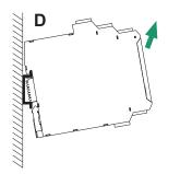
D. Remove the safety barrier as arrow shows.O As far as possible to mount it vertically, In order to dissipation the heat of the apparatus.
