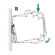
B. Snap metal lock onto mounting rail, then rotate the safety barrier, as figure B, press down the safety barrier onto mounting rail, make sure that the BUS connector pins of safety barrier and BUS socket are in close contact.
