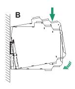
B. Snap metal lock onto mounting rail, then rotate the safety barrier, as figure B, press down the safety barrier onto mounting rail, make sure that the BUS connector pins of safety barrier and BUS socket are in close contact.
