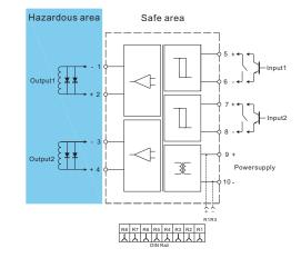
O DIN rail power supply function is selectable at ordering.
