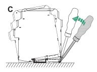
C. Pry the metal lock off the rail with screwdriver as arrow shown, pull downward the springs, and rotate the apparatus.
