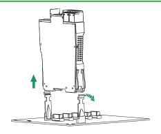
Pull the slot of the backplans outward, and remove the apparatus as arrow shows .
