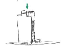
Install the apparatus, make the both sides of the apparatus aim at the slot of the backplans, press down the apparatus onto the backplans as the direction of the arrow.
