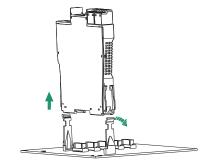
Pull the slot of the backplans outward, and remove the apparatus as arrow shows .
