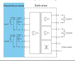
O Follow mode: Whatever input fault status (except breakage, the output value is 0 V/mA), the output follows the input within measuring range. And the maximum value would not exceed the 110% of the upper limit of the measuring range (e.g. When the output signal type is 0 ~ 20 mA, the minimum output value may be 0 mA, the maximum output value would not exceed 22 mA).
