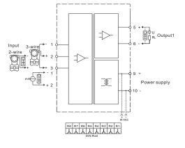
Single current input, double sink mode output
