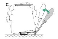
C. Pry the metal lock off the rail with screwdriver as arrow shown, pull downward the springs, and rotate the devices.
