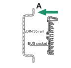
O A. Snap the BUS socket on the DIN 35 rail, as figure A;
