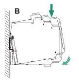
B. Snap metal lock onto mounting rail, then rotate the devices, as figure B, press down the devices onto mounting rail, make sure that the BUS connector pins of devices and BUS socket are in close contact.
