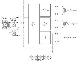
Single voltage input, single current/voltage output
